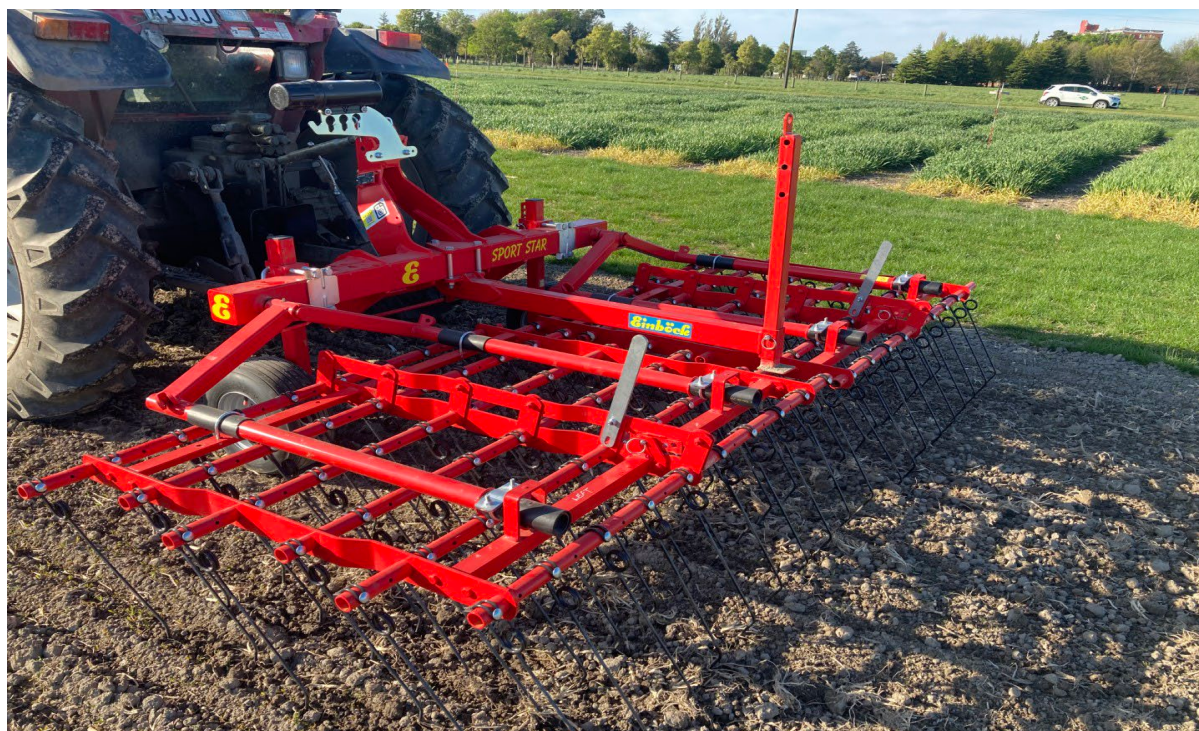
Figure 4. Three metre wide Einböck AEROSTAR-CLASSIC spring tine weeder used in the barley autumn and spring weed control trial at Kowhai, Lincoln in 2023-24.
