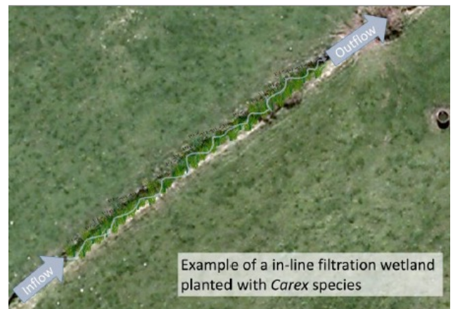
Figure 17. In-line filtration wetlands (Image source: Wai Kōkopu Consulting).
