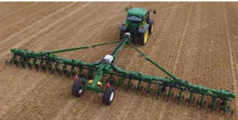
Figure 31. Roe-hoe consisting of a number of independent parallelogram units mounted on a toolbar. Right photo Garford Farm Machinery Ltd.
