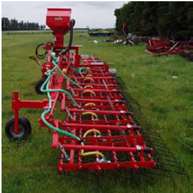
Figure 28. Spring tine weeder with pneumatic seeder.
