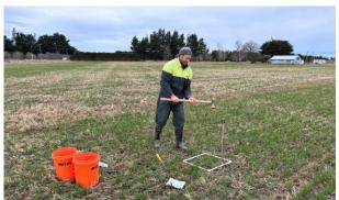
the ground conditions were perfect for getting the soil probe hammered in. If this prompts you to think about beginning soil testing yourself, a useful resource can be found <u>here</u>. Also see our article on a quick soil testing method <u>below</u>.
